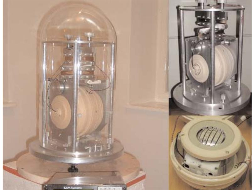
dIdD integrated 3 component coil system with enclosed Overhauser sensor designed for long-term observatory monitoring applications.
